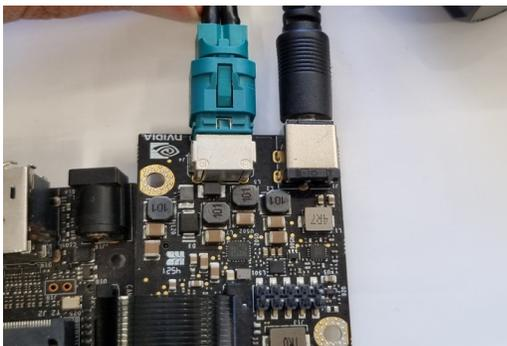
Once cables are connected, plug the power for the GMSL2 capture card (12V-19V) so that cameras will be powered through the FAKRA cable (PoC).
