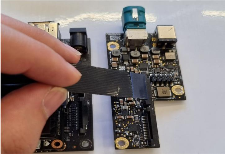
**Warning :** Inverting the side might damage the carrier board or the capture card
